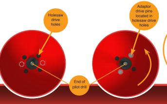
If the holesaw is turned in the direction of the arrow, the drive pins can be located in the first pair of drive holes they arrive at.
